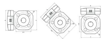
Horizontal installation with counter showing sideways (preferred), 45 °C up (recommended minimum) and upwards (not recommended)
