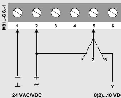
Override control of M91..GG.-1 actuators can be provided with the circuitry shown opposite.
