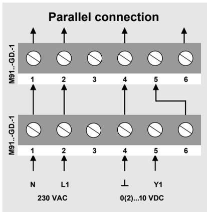
When M91..-GD.-1 actuators are to be operated in parallel, the output signal U = 0(2)...10 VDC (Terminal 6) of the master actuator must be connected to Terminal 5 of the next slave actuator, etc.
