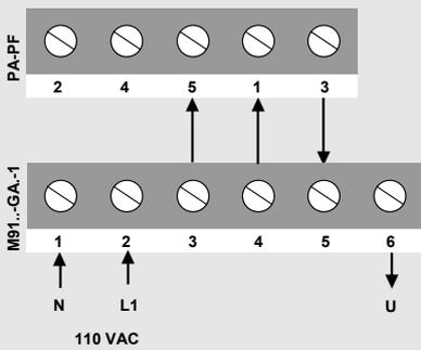
M91..GA.-1 actuators can also be controlled by means of a Johnson Controls M9000-PA/PF remote positioner with 0(2)...10 VDC control signal.
