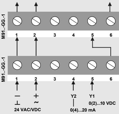
When M91..GG.-1 actuators are to be operated in parallel, the output signal U = 0(2)...10 VDC (Terminal 6) of the master actuator must be connected to Terminal 5 of the next slave actuator, etc.
