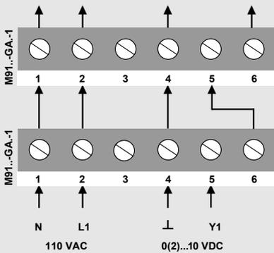
When M91..GA.-1 actuators are to be operated in parallel, the output signal U = 0(2)...10 VDC (Terminal 6) of the master actuator must be connected to Terminal 5 of the next slave actuator, etc.
