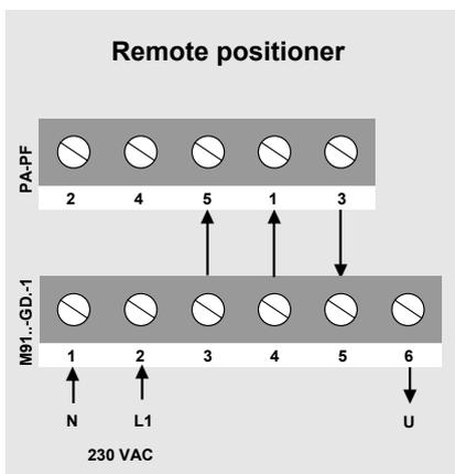
M91..-GD.-1 actuators can also be controlled by means of a Johnson Controls M9000-PA/PF remote positioner with 0(2)...10 VDC control signal.
