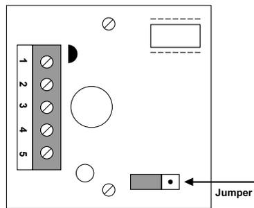
The output signal 0...10 VDC or 2...10 VDC ist proportional to 0...100% rotation of the adjuster knob.
