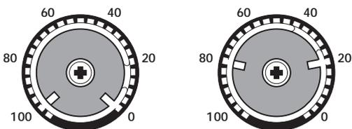
The adjuster knob can be removed by pulling it out of the front plate. Inside the knob the mechanical limiting of the angle-of-rotation can be adjusted by moving the stop springs.
