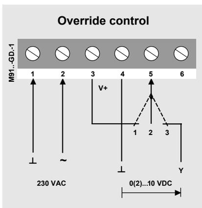
Override control of M91..-GD.-1 actuators can be provided with the circuitry shown opposite.
