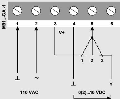
Override control of M91..GA.-1 actuators can be provided with the circuitry shown opposite.
