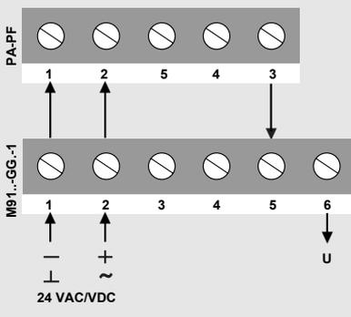
M91..GG.-1 actuators can also be controlled by means of a Johnson Controls M9000-PA/PF remote positioner with 0(2)...10 VDC control signal.
