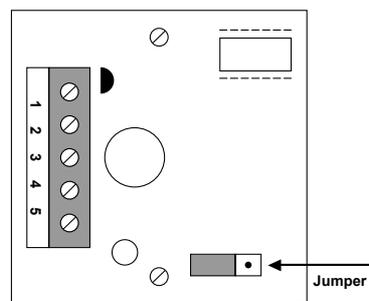
The output signal 0...10 VDC or 2...10 VDC is proportional to 0...100% rotation of the adjuster knob.
